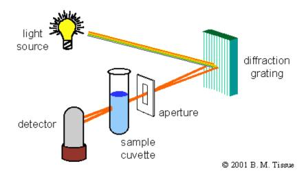
**Figure 1. Schematic of a single-beam UV-Vis spectrophotometer**. Image available at http://www.files.chem.vt.edu/chem-ed/spec/uv-vis/singlebeam.html
